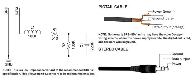
Figure 2 Equivalent circuit diagram
