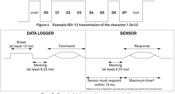
Figure 5 Example data logger and sensor communication
